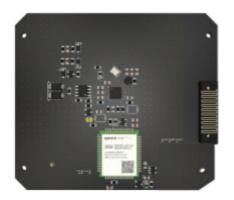
IoT is an advanced and value engineered hardware solution for the Internet- of-Things (IoT). It includes basic features such as GPS and accelerometer as well as advanced CAN communication protocol and over-the-air (OTA) updates. Additionally, it features intelligent onboard software algorithms for movement detection, crash detection, hard
